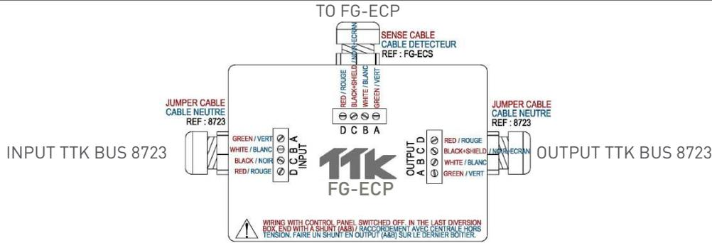
FG-ECP is made of Four Wires Sense Cable FG-ECS:
