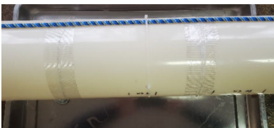
The sense cable is fastened on the side of the pipe base.
