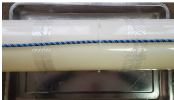
The sense cable is fastened at the 6 o'clock position beneath the pipe, positioned centrally under the pipe. (The photo is captured from beneath the pipe)
